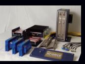
The NHANCE Control System uses the latest technology to allow aging DC and SW locomotives to be upgraded to a level of performance matching that of their modern counterparts. The system is designed for fouraxle locomotives using the 74V batteries to excite the Main Generator, providing consistent locomotive performance, increased reliability through reduction in high maintenance components and greatly improved all weather tractive effort.
